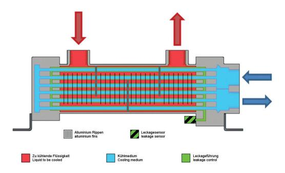
Based on their existing hybrid heat exchangers from the SCM-Series, Universal Hydraulik developed a new high efficiency fail-safe heat exchanger, the SCM/FS. The advantages of the hybrid design, such as a compact size or an internal bypass valve of the newest generation, can be completely utilized.
